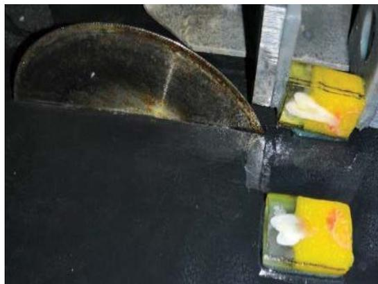
Figure 1: Specimen sectioning with microtome.
