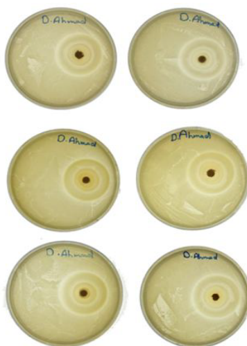
Figure 12: New gutta percha showing the inhibition zone.
