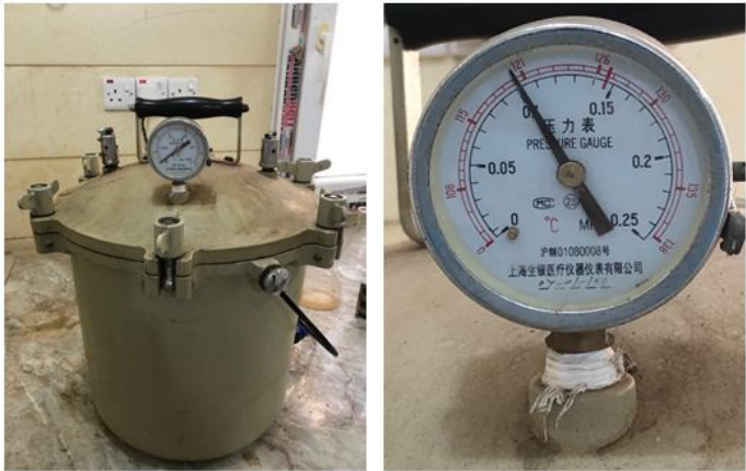
Figure 6: Pressure up gradually to 121 PSI.
