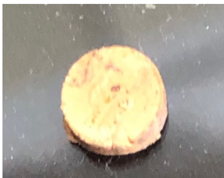
Figure 3: Disc of gutta percha (0.035 grms) with 5mm width and 2mm height.
