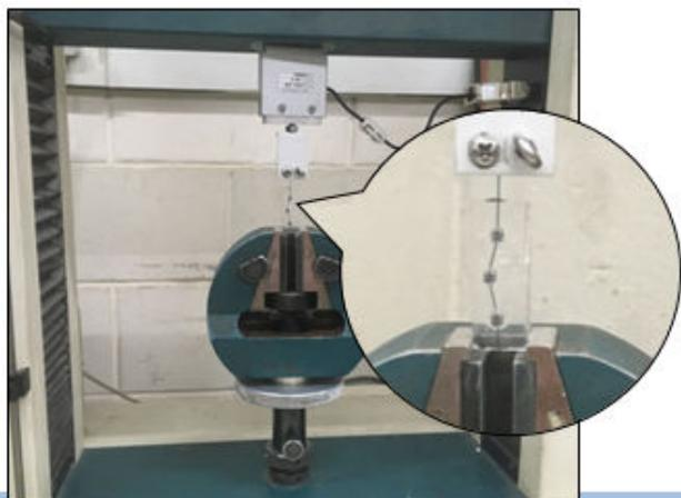
**Figure 1: Specimen of the test attached to 10 N load cell of Instron tinius olsen universal testing machine to test frictional resistance.**
