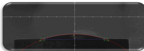
Figure 2: Measurement of water titanium disk contact angle.
