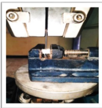
Figure 1: Instron universal testing Machine with bone/implant block.
