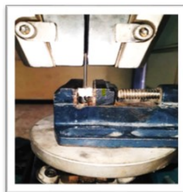
Figure 1: Instron universal testing Machine with bone/implant block.
