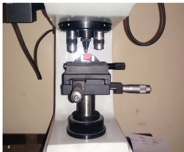
Figure 2: Specimens loaded for Vickers microhardness test 50 grams for 10 seconds.
