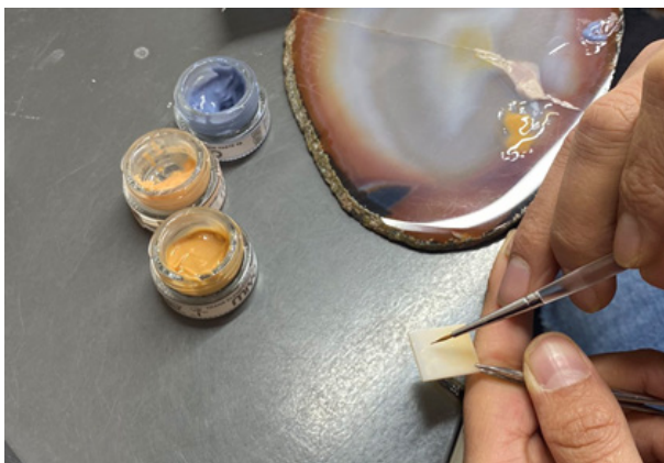
Figure 2: Application of MiYO colors to monolithic zirconia specimens.
