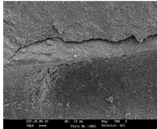
**Figure 9:** SEM image of bonding micro hybrid and micro hybrid composites using silane-bonding as the interfacial material
