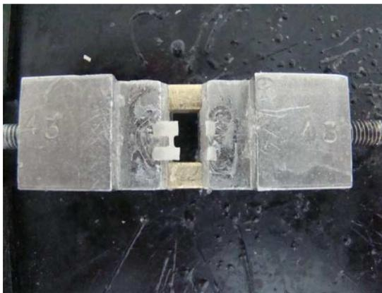
**Figure 7:** Bonding of nano hybrid and micro hybrid composites together with the cohesive fracture
