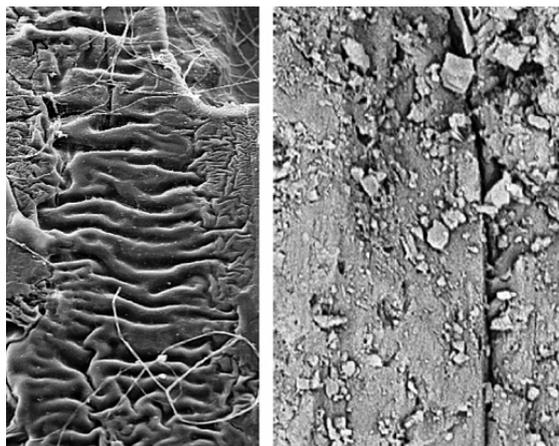
**Figure 8:** SEM image of bonding micro hybrid and micro hybrid composites using a composite flow as the interfacial material
