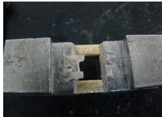
**Figure 10:** Bonding micro hybrid and micro hybrid composites together with the cohesive fracture
