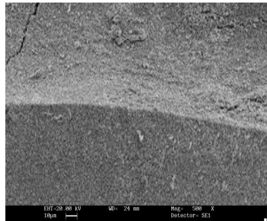
**Figure 3: SEM image of bonding nano hybrid and nano hybrid composites using silane-bonding**
