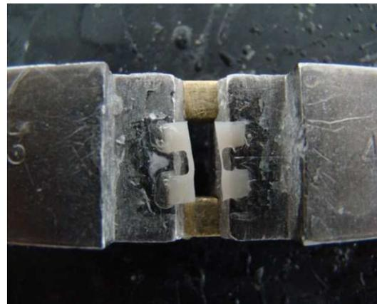
**Figure 4: The image of bonding nano hybrid and nano hybrid composites separated from the bonded area**
