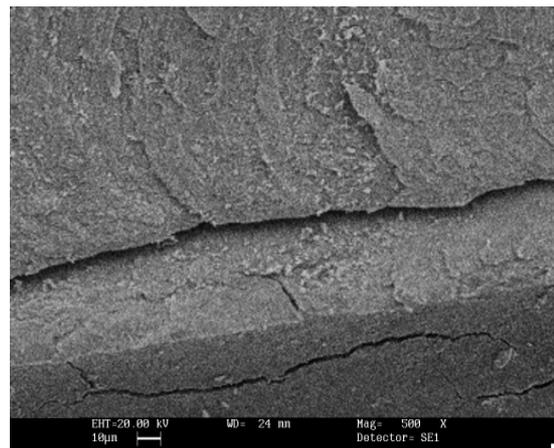
**Figure 5: SEM image of bonding nano hybrid and micro hybrid composites using a composite flow**
