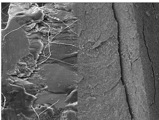
**Figure 2: SEM image of bonding nano hybrid and nano hybrid composites using a composite flow**
