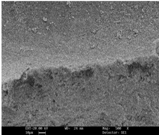
**Figure 6:** SEM image of bonding nano hybrid and micro hybrid composites using silane-bonding
