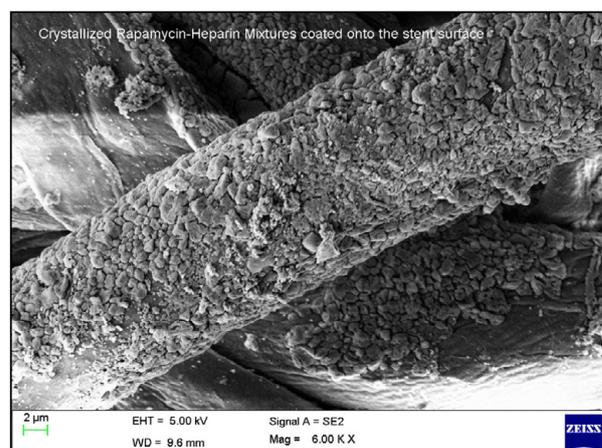
Figure 1: FESEM analysis of drug and carrier-coated coronary stents.
