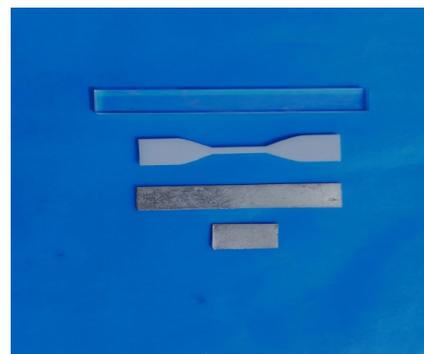
Figure 1: A, plastic mold for impact test. B, plastic mold for elongation test. C, metal mold for hardness and roughness test. D, metal mold for color stability test.
