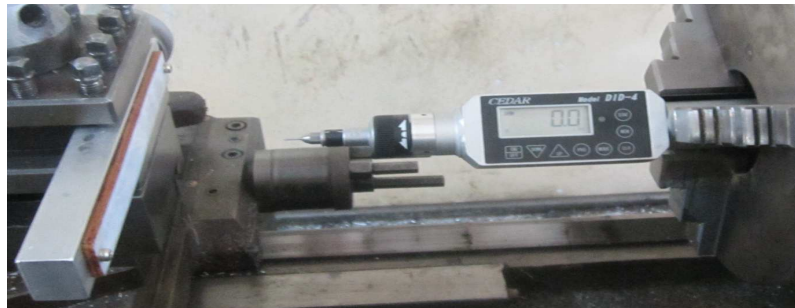
Figure 1. Mini-screw was placed by a custom made screw driver on Imada torque tester which was clasp in milling machine. With rotational movement of milling machine mini-screw was inserted to polycarbonate plate, and Imada torque tester showed torque values.
