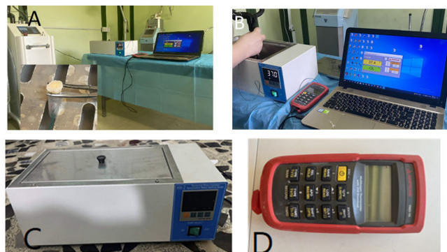
Figure 5: A) Set up for temperature measurement in the tooth pulp during laser radiation, thermocouple inserted inside pulp chamber; B) Thermometer records rise in temperature during lasing; C) Water bath use to allow the temperature to reach 37°C; D) Thermometer.
