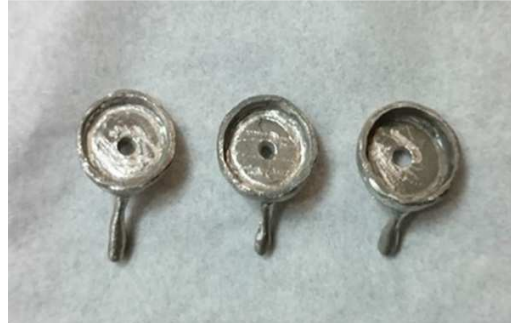
Figure 1: Metal molds for standardization of lithium disilicate core thickness
