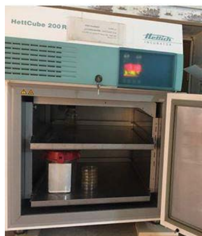
Figure 4: Incubator for incubation anaerobic bacteria with gas pack in an anaerobic jar.
