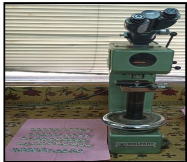
Figure 3: Teeth sample were measured by Vickers micro-hardness testing machine.
