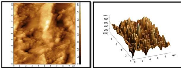
**Figure 2:** After treatment with NHA GEL: A uniform and homogeneous coating with a smooth surface and more particles and grain, with some lightness and dark area visible in on surface locations. But whiter than the same sample in the previous stage.
