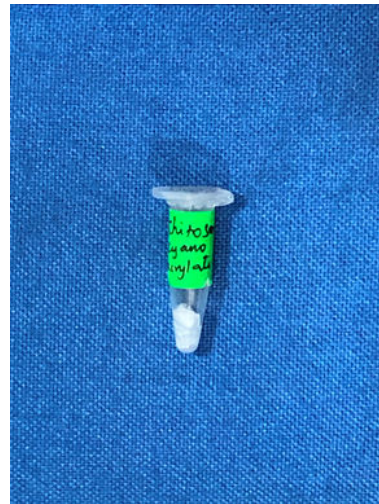
Figure 4: Cyanoacrylate infused with chitosan.
