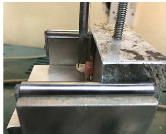
Figure 4: Bond strength testing
