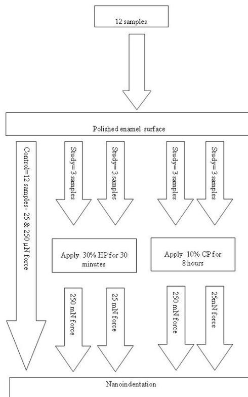
**Figure 4: Showing the experimental outline for nanoindentation tests before and after dental bleaching**
