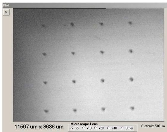
**Figure 2: Showing Indentation tests on an enamel surface before application of the dental bleaching agent at a force of 250 mN. Microscopic image (5x) of one of the enamel samples showing the indentations with a distance of 100 µm between the indents.**
