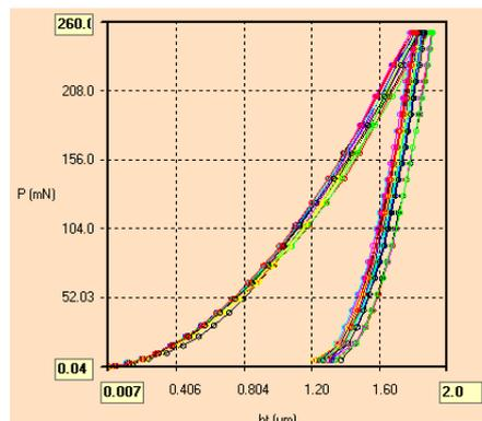
Figure 5: Showing Examples of a load displacement (P-h) curve with a nanoindentation test using 250 mN and control enamel. The x-axis represents the displacement, and the y-axis represents the load. The results of 16 indentations are shown on the graph.
