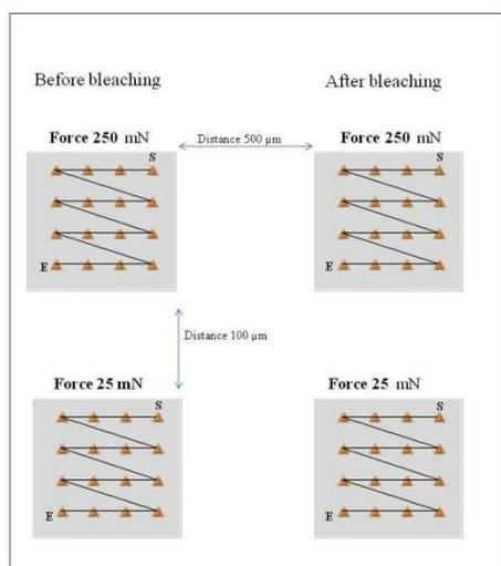
**Figure 3: Showing the testing procedures for each sample. The line (S→N) indicates the path that the nanoindenter took in making the indentation (shown as triangles) in the samples. S= Starting point for the test; E=End point**
