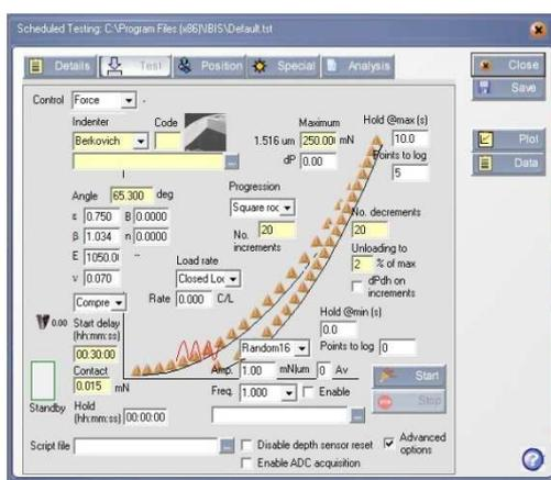
**Figure 1: Showing the nanoindentation settings for testing with a 250mN force.**
