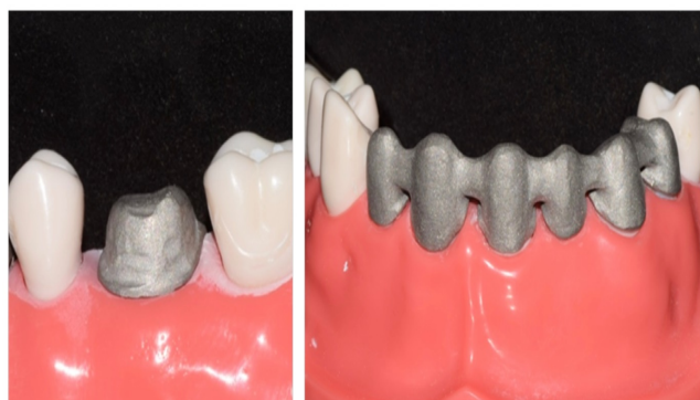
Figure 2: Pictorial representation of the anterior and posterior prosthesis fabricated after the DMLS printing.
