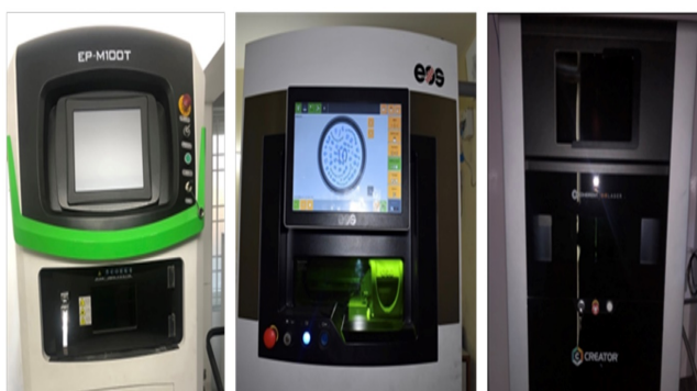
Figure 1: Pictorial representation of the three machines used to fabricate the dmlls prosthesis (EOS M 100, Shining 3D EP-M 100T and OR laser Creator machine).
