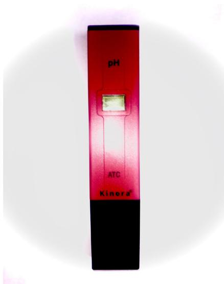
Figure 2: Shows the Pocket Digital pH meter (manufactured by KINORA). It has a range of 0.0 to 14.0 with an accuracy of + 0.1 pH and accuracy of  $\pm 0.1$ pH. The device is calibrated before each use and was covered using protective cap after every use to prevent miscalibration.
