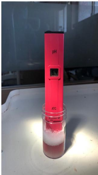
Figure 3: Image shows the salivary sample pH being assessed immediately after collection using the device (Kinora pH digital meter) with the tip of the electrode completely immersed into the sample. The pH value of 6.4 is shown on the display.
