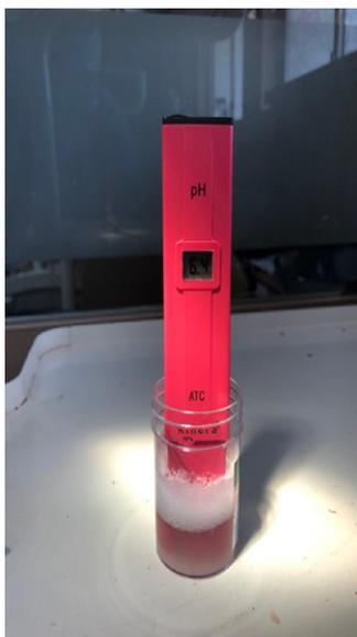
Figure 3: Image shows the salivary sample pH being assessed immediately after collection using the device (Kinora pH digital meter) with the tip of the electrode completely immersed into the sample. The pH value of 6.4 is shown on the display.
