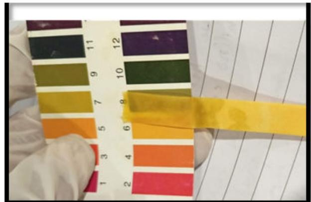
**Figure 4: Comparing change in colour with standard pH scale.**
