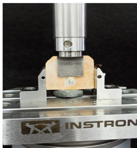
Figure 2: Sample loaded in a universal testing machine (Instron).
