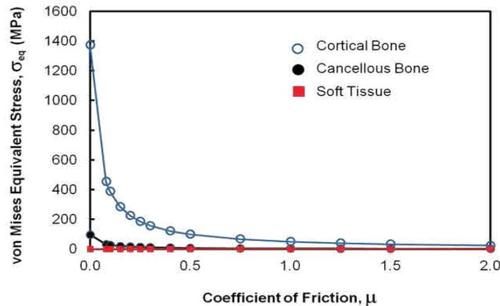
Figure 5: Maximum von Mises equivalent stress plotted against the coefficient of friction  $\mu$ .
