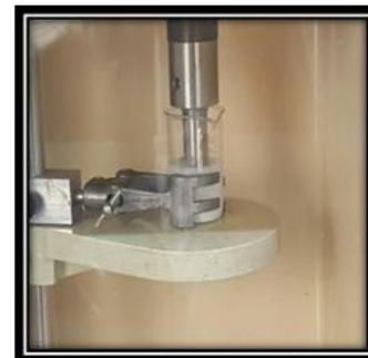
Figure 1B: Probe sonication apparatus.
