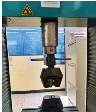
Figure 5: The computer-controlled universal testing machine used in the study.
