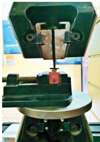
Figure 6: Representation of rod application used for axial compression test: The tooth with its acrylic block fixed to the base of the testing machine.
