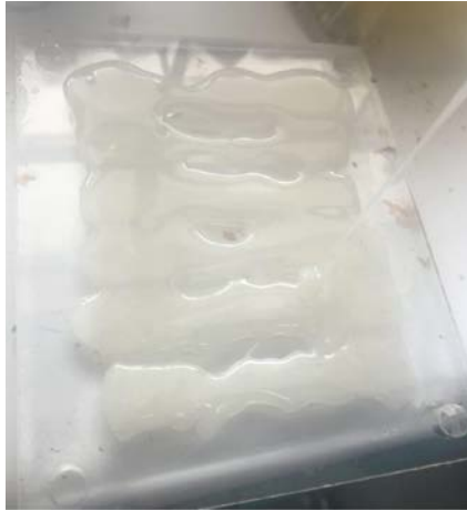
Figure 2: Filling mold with silicone material
