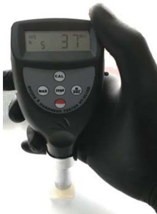
Figure 4: Shore A durometer used to measure hardness of silicone sample
