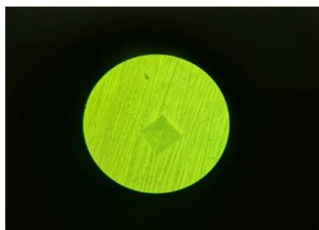
**Figure (7): a) A schematic illustration of Vickers technique (Vickers microhardness machine utilizes a 136° diamond pyramid indenter that forms a square indent on the surface. b) An image taken by the researcher of a tetra pyramidal indentation in Vickers technique that creates a clear, measurable indentation in the field as diagonals.**
