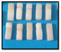
Figure 4: Shear bond samples substructure clear heat cure and veneer IPS E-max ceramic joint to gather by using Glass ionomer cement.
