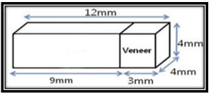
Figure 1: Dimension of shear bond strength sample.
