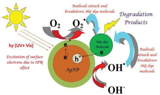
Figure 2: Mechanism of MG dye degradation utilizing photocatalytic AgNPs synthesized from CN extract and activated by sun light [7].
