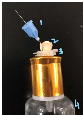
Figure 1: Experimental model showing its components 1-needle; 2- tooth; 3-eppendorf's tube and 4-glass vial.
