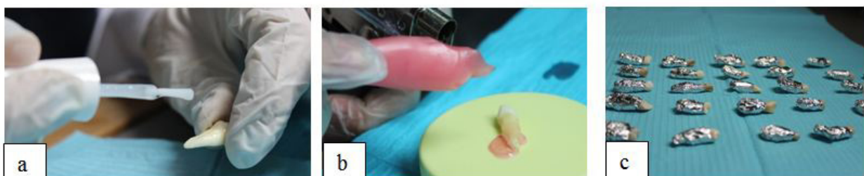
Figure 1: (a) Teeth coated with three layers; (b): Wax melted over the roots; (c) Aluminium foil as the last seal of clear varnish.
