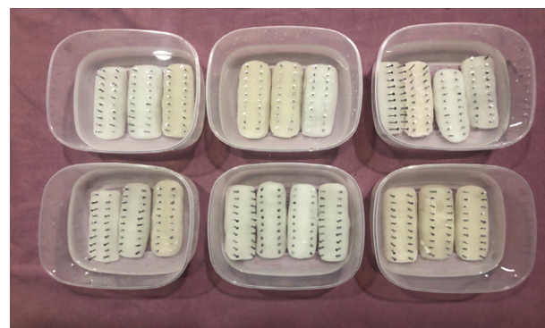
Figure 2: Elastomeric chains held between the pins of acrylic boards and immersed in artificial saliva.
