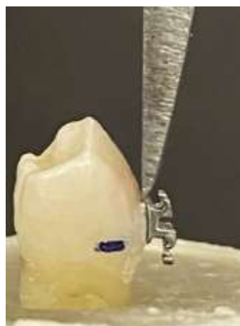
Figure 4: Photograph showing the position of the knife-edge portion of the Instron machine as being perpendicular to the bracket-tooth interface.
