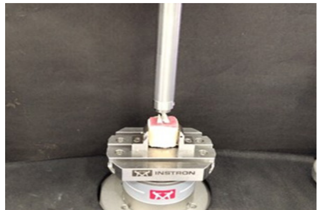
Figure 6: Shows the mounted tooth with fibre splint to detect the flexural strength.
