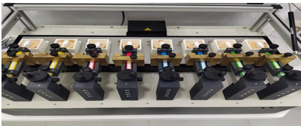
Figure 5: Shows the mounted tooth model of Interlig and Techno fibre splint placed in toothbrush simulator.
