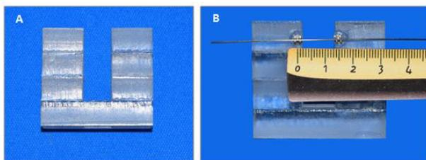
Figure 2: A, Custom made U-shape acrylic block; B, 0.022 slot brackets bonded to the block with aid of 0.021 x 0.025-in SS wire.
