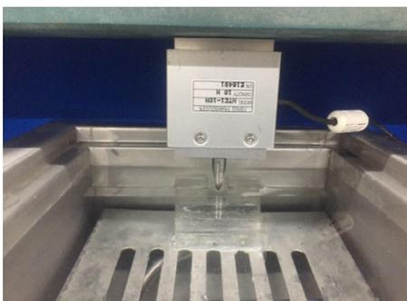
Figure 3: Modified load deflection bending test of archwire segment.
