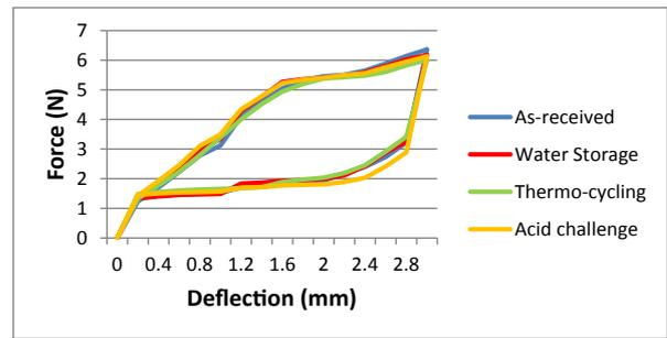
Figure 4: Load deflection curves for 0.016 inch Niti arch wires in as-received and artificial aging conditions.
