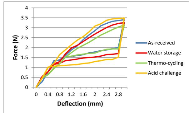
Figure 5: Load deflection curves for 0.016 inch CuNiti archwires in as-received and artificial aging conditions.
