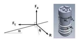
Figure 1: Forces and moments acting on the screw on its tightening.
