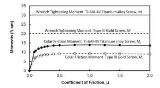
Figure 3: Moment Mc for the screw materials of Ti-6Al-4V titanium alloy and type III gold versus the coefficient of friction  $\mu$  as calculated by equation 5.
