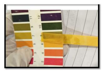
Figure 4: Comparing change in colour with standard pH scale.
