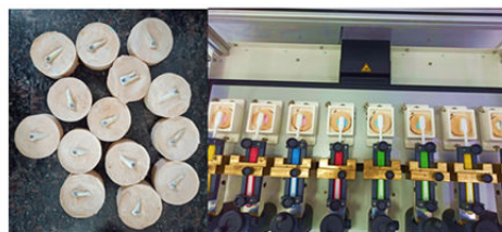
Figure 1a: Samples mounted in die stone; b) Samples loaded in a brushing simulator.
