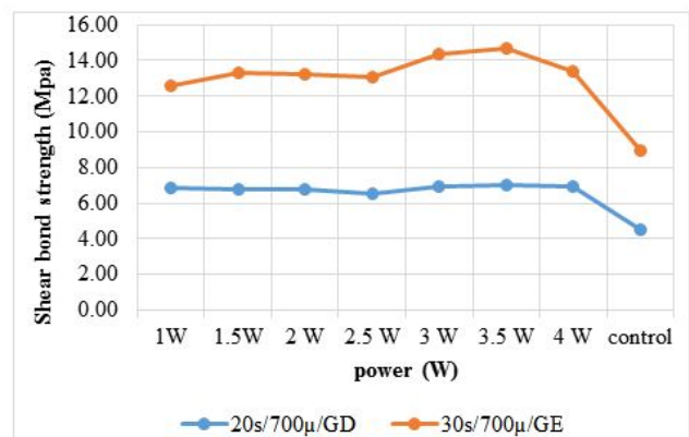
Figure 7B: The shear bond strength as a function of Er,Cr:YSGG laser power for groups related to(700 µs) pulse duration (Group D/20s, 700µs. Group E/30s, 700µs).
