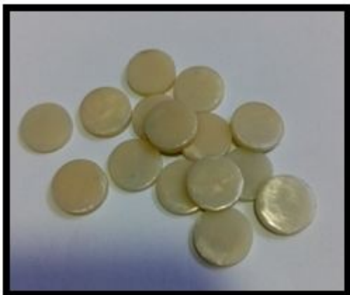
Figure 2: CAD-CAM milled zirconia samples.
