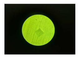
Figure (7): a) A schematic illustration of Vickers technique (Vickers microhardness machine utilizes a 136° diamond pyramid indenter that forms a square indent on the surface. b) An image taken by the researcher of a tetra pyramidal indentation in Vickers technique that creates a clear, measurable indentation in the field as diagonals.
