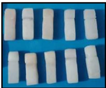
Figure 3: Shear bond samples substructure clear heat cure and veneer IPS E-max ceramic joint to gather by using Breeze self-adhesive resin cement.
