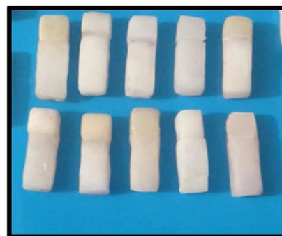
Figure 4: Shear bond samples substructure clear heat cure and veneer IPS E-max ceramic joint to gather by using Glass ionomer cement.
