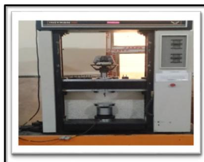
Figure 5: Instron-1195 testing machine, the sample in holder and mounted in a universal testing machine.
